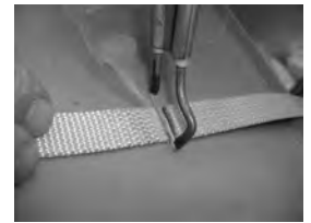
Cut the webbing with a heat cutter.
