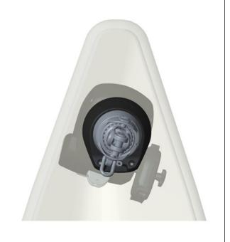
Fit the swivel through the deck fitting and motor unit.
