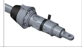
Remove clevis pin and split pin from motor unit and slide the motor unit over the swivel.
