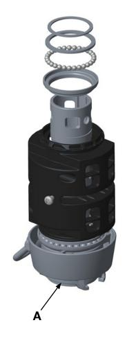
With a firm grip of the tack ring (B), wiggle and lift the line drum.
